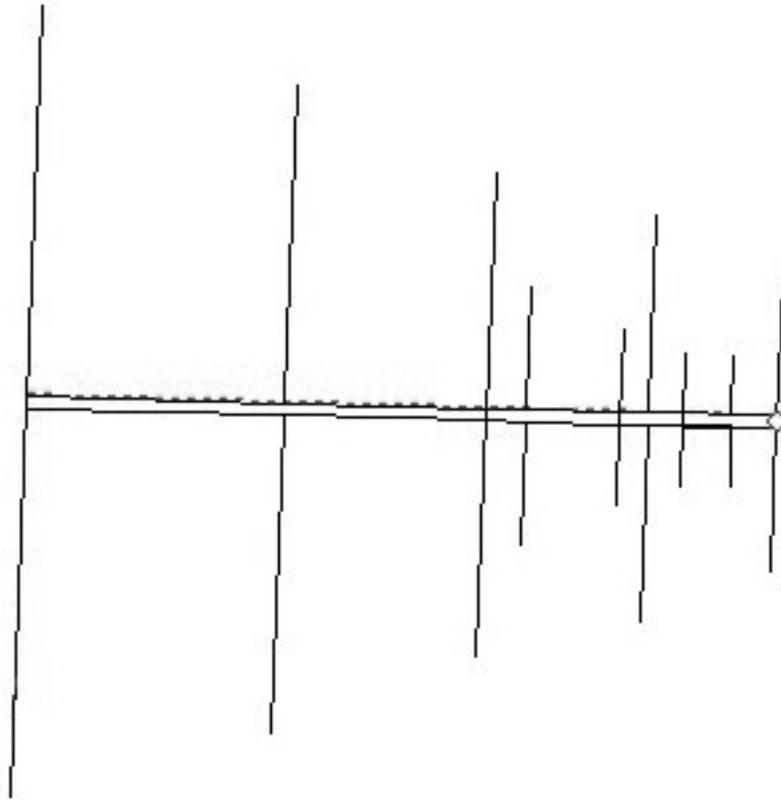
Table of elements starting with the longest element. Feed 3/16" diameter space 7/32" center to center, elements 1/16" diameter.
