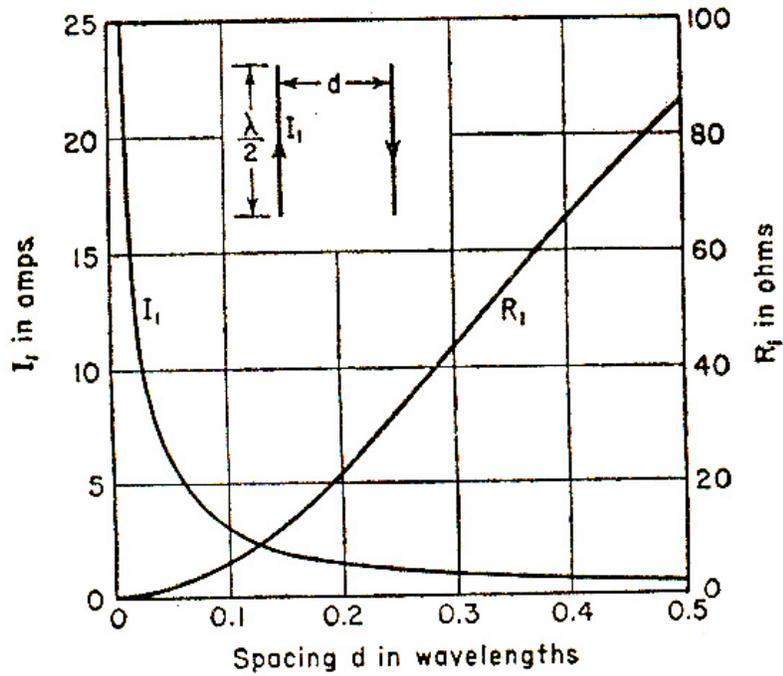
FIG. 11-15. Current  $I_1$  and radiation resistance  $R_1$  in each element of a flat-top beam antenna as a function of the spacing. The current is calculated for a constant input power of 100 watts to the array.
