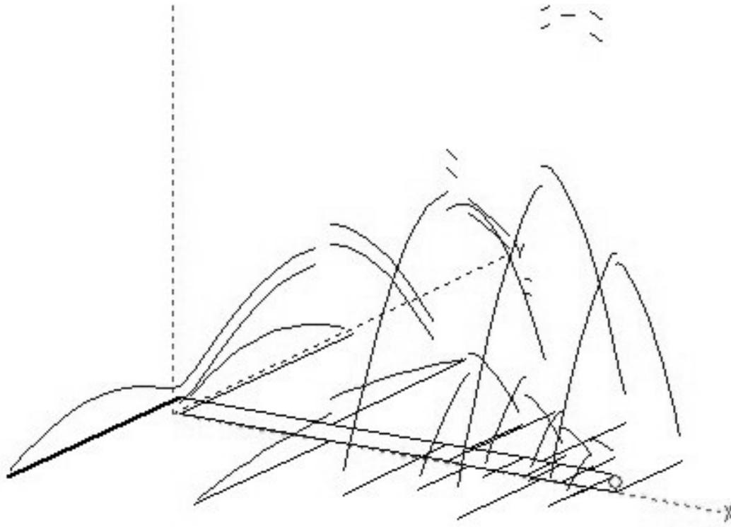
Element currents of the KØCQ short feet at 1296, and the radiation patterns.
