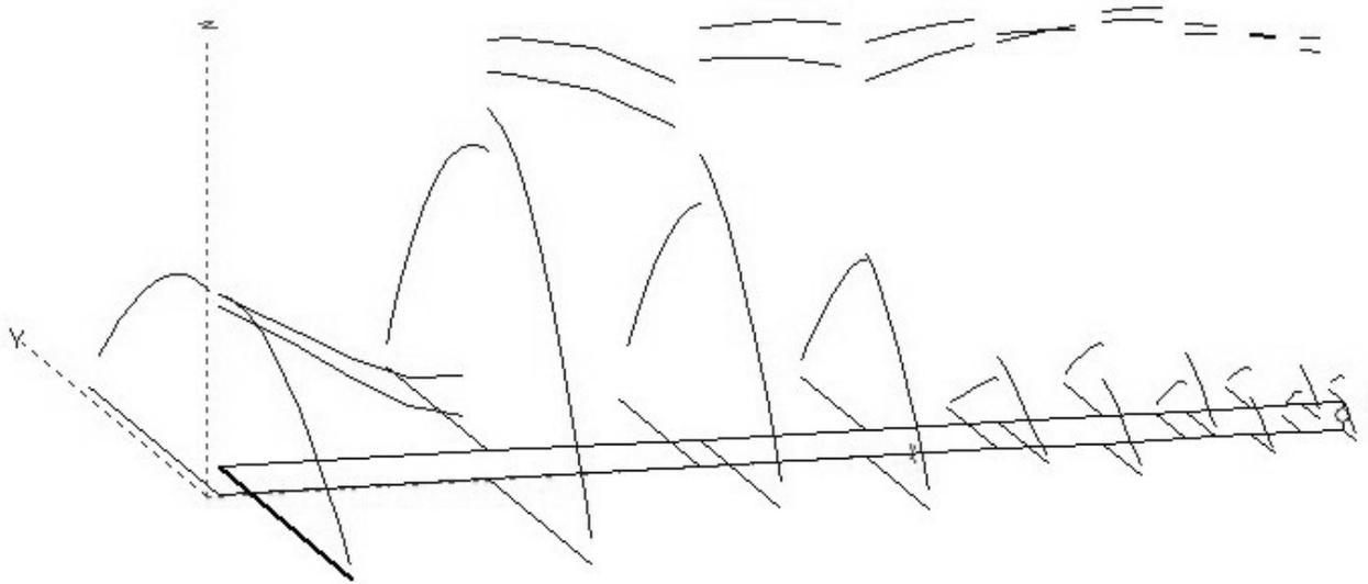
This is the Mmana-Gal current display of Ben's feed at 902 MHz. And it gives a computed radiation pattern next.
