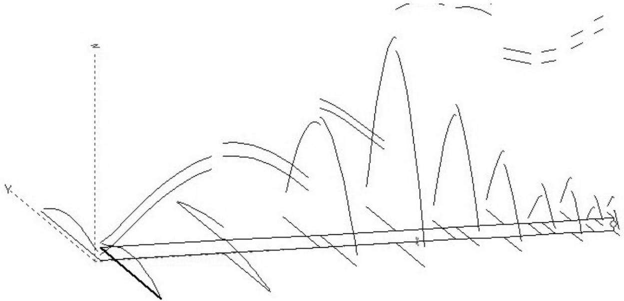
This is the current plot for 1296. Notice the feed current between elements 4 and 5 is greater than the element currents. A sign of W8JK mode of close spaced elements fed out of phase where the coupling raises the currents in the elements and so give some gain.
