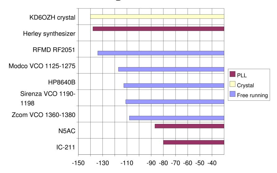
Noise dBc/Hz for 10 KHz offset at 1 to 1.2 GHz
