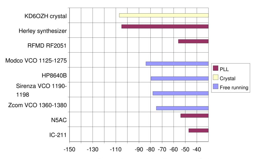
Noise dBc/Hz for 10 KHz offset at 47 GHz
