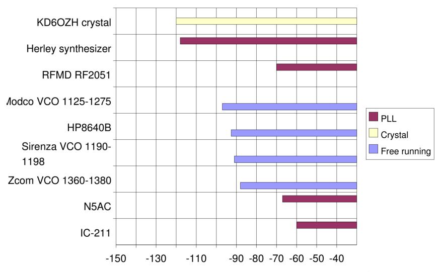
Noise dBc/Hz for 10 KHz offset at 10 to 12 GHz
