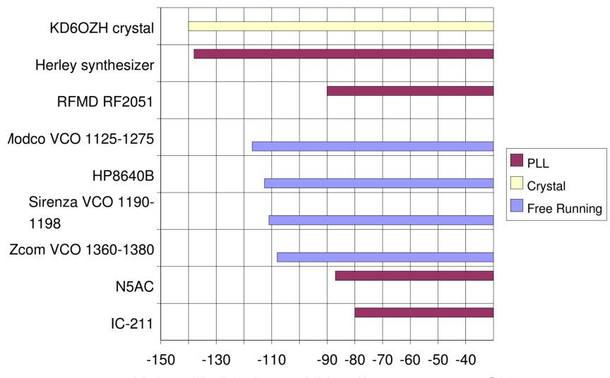
Noise dBc/Hz for 10 KHz offset at 1 to 1.2 GHz
